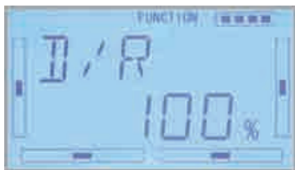
(3) Dual Rate adjustment
